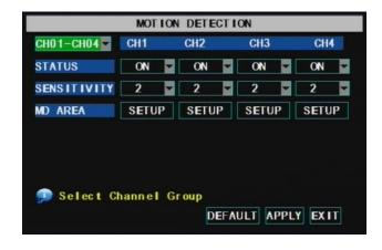
Next, click on the MD AREA SETUP button, which will display the picture on the left. This option allows you to select the area you want to be sensitive to motion. The area in red is sensitive to motion. You can set this area by using the mouse or REV, FWD, and SEL keys on the front panel. Once you have set the area, right click with the mouse or push the ESC key to save the setting. After you have set all of the cameras, click on the Apply button to save the settings.
